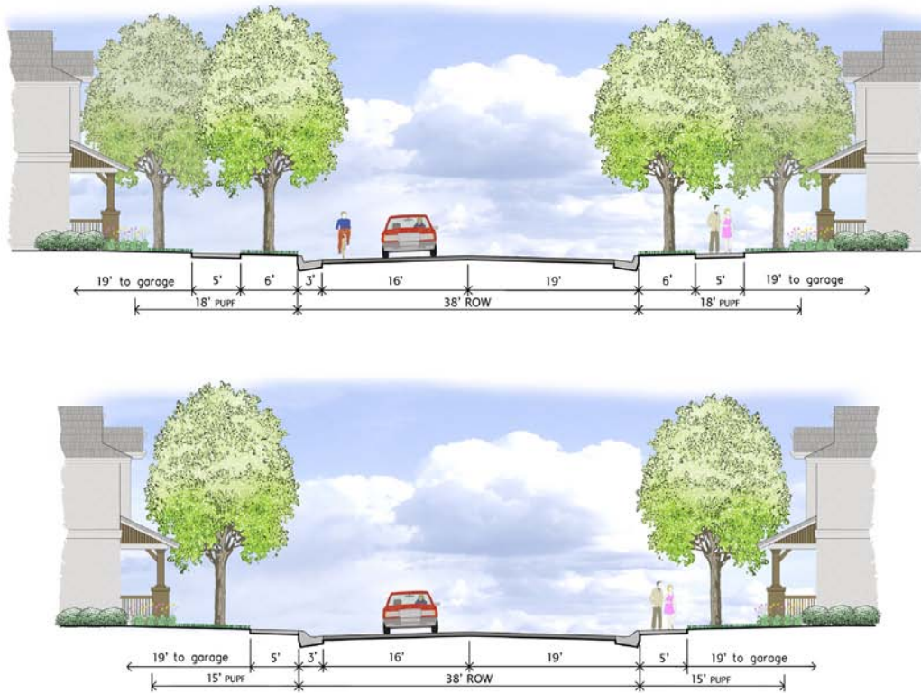
Figure 9.6 Primary Residential - Separated and Attached Walk
