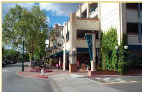
Parking structures should be designed with ground-floor retail or office to add character to a street and to avoid blank walls.
