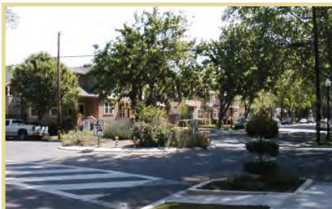
Traffic circles are raised islands in the intersection.
