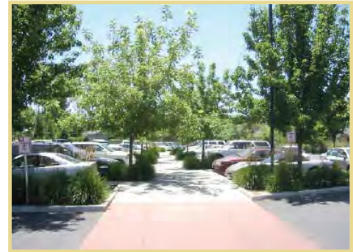
Parking lots should minimize conflicts between pedestrians and traffic by identifying separate pedestrian and vehicular circulation routes.
