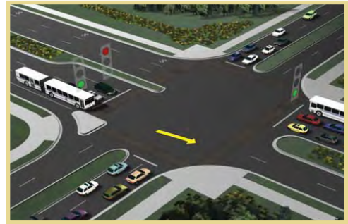
Transit preemption allows buses to continue through an intersection while regular traffic is stopped.
