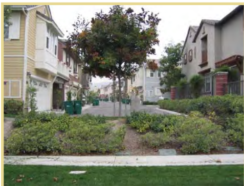
Creative site solutions and building arrangements, such as enhanced landscape buffers, are encouraged along high-traffic streets to avoid the use of sound walls.
