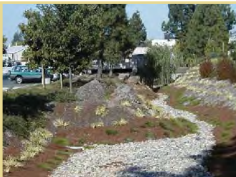
Bioswales and other opportunities to incorporate energy and water efficient landscaping and drainage practices should be promoted.
