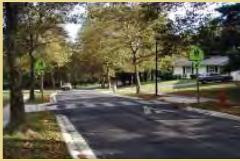
Speed tables are flat-topped speed bumps used to slow traffic.
