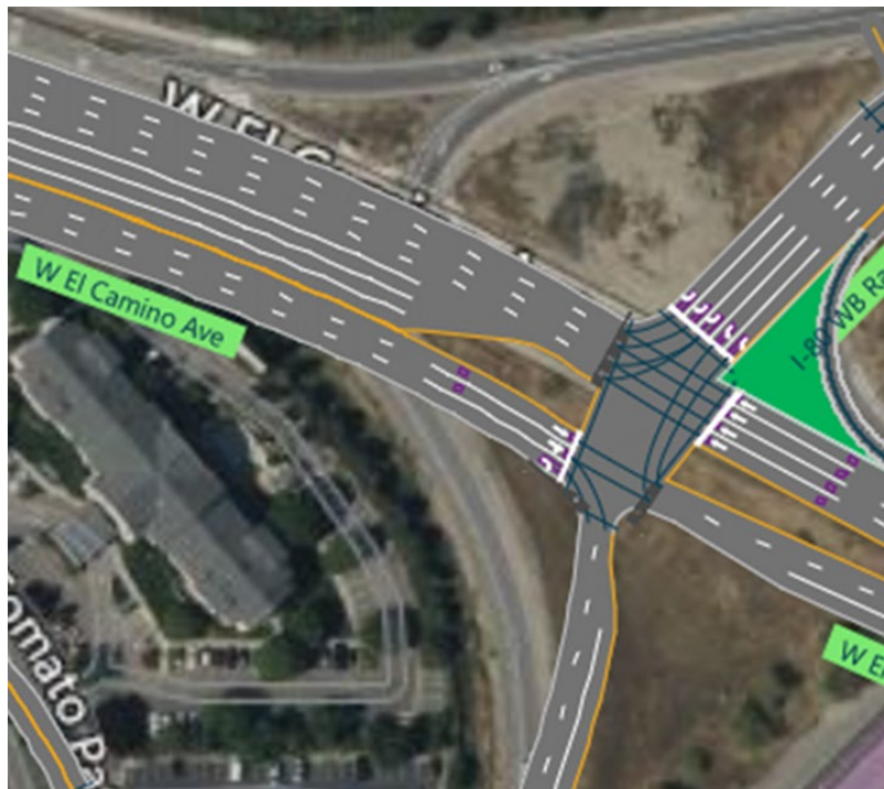
Image 4: SimTraffic screenshot showing final geometrics recommended for the I-80 Westbound Ramps/West El Camino Avenue intersection.
